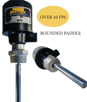
This construction is ideal for violent flows or heavy paddles. We also offer a pivot at the base of the switch, with the stem and paddle hanging on this pivot. Above the pivot, the stem ends in a socket which operates a ball attached to the upper stem.
