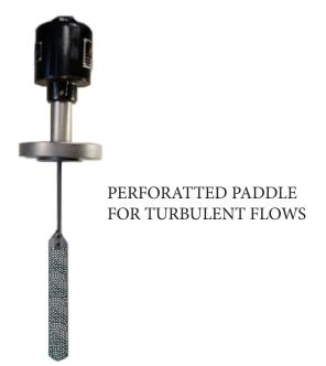
The symmetrically placed perforations help reduce turbulence and cavitation. Excessive turbulence and build-up of vacuum behind the paddle is prevented.
