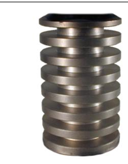
Supplied with a variable length of convoluted stainless steel body extension permitting rapid-heat dissipation. This inhibits the high heat from passing through the body and into the electrical components located in the topworks.
